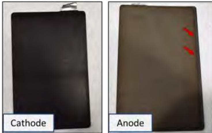
Cell Disassembly – Cell Discharged @ 0.2C @ 60°C
