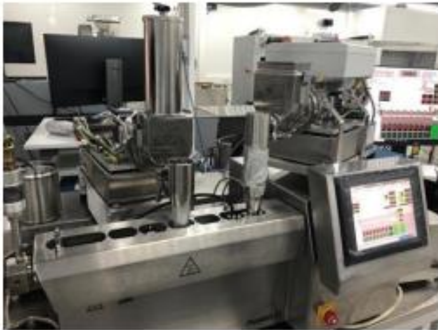
+ Equipment: Pharma11 (ThermoScientific), 11 mm diameter, L/D=40
