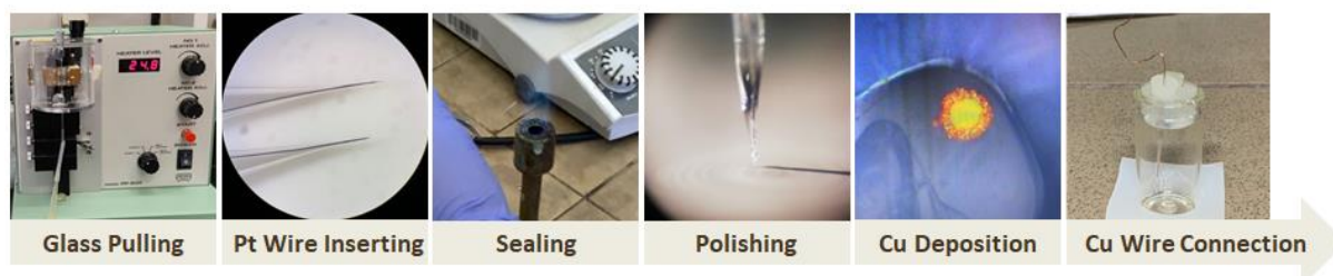
Figure 8 Main steps of preparing a microelectrode in the lab
