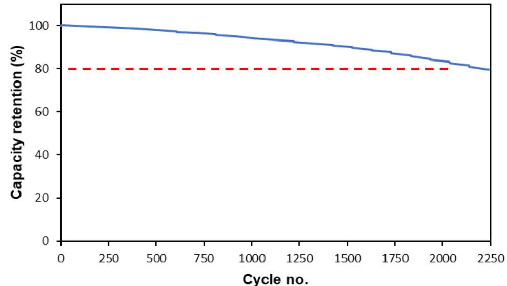
+ Full-cell cycle tests show promising results with **80% capacity retention after 2241 cycles**
